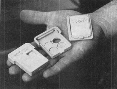
DISASSEMBLED FILM BADGE shows three filters and code on film visible when film is properly placed in new plastic holder.
